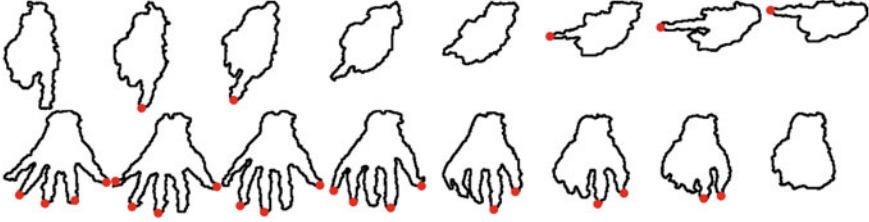
Fig. 14.6 2D shape features defined on hand contour. The red points indicate the locations of features
