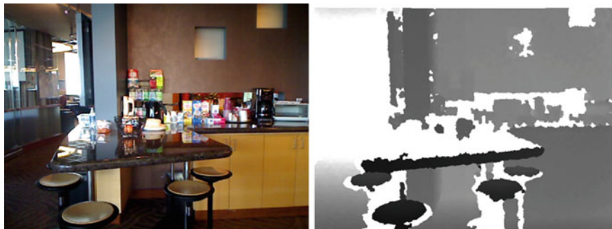
Fig. 1.12 Artifacts commonly occur in depth capture of natural scenes using commercial 3D cameras. Left RGB image. Right Depth map captured by the first-generation Kinect of the same scene. Pixels in white are holes in the depth map which arise due to specularities occlusion or clutter. Image courtesy [9]
