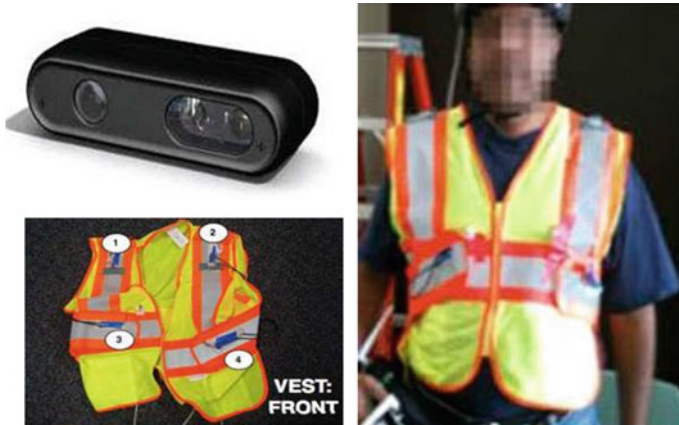
Fig. 9.6 The RGB-D camera-based navigation aid for the visually impaired, which includes an RGB-D camera and a tactile vest interface device [52]
