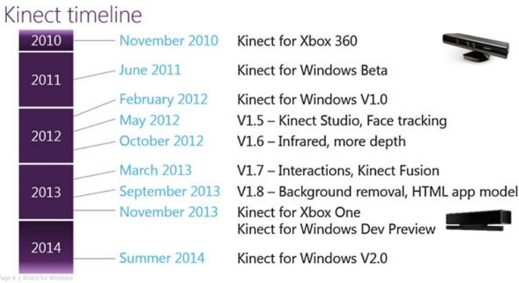
Fig. 1.18 Time line of the Kinect projects. The structured light Kinect was released in 2010, while the time-of-flight Kinect was released in 2013. Graphic courtesy John Elsbree
