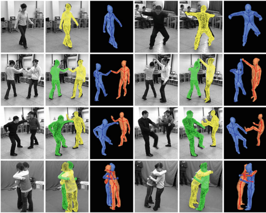
Fig. 5.4 Performance capture results on a variety of sequences: one of the input image, layered geometry, reconstructed geometry, and skeleton. Each row shows two results
