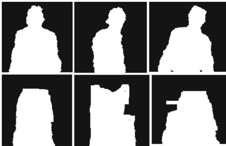
Fig. 10.6 Training samples for human detection. Top the positive samples. Bottom the negative samples
