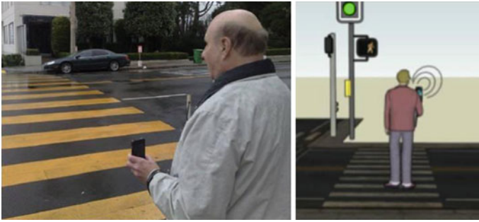
Fig. 9.2 Crosswalk system for providing guidance to visually impaired pedestrians at traffic intersections by panning a cell phone camera left and right ; the system provides feedback to help user align him/herself to crosswalk before entering it [28]
