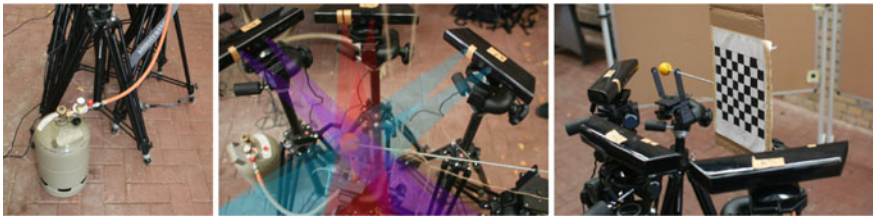
Fig. 8.1 We examine small pixel deviations in the IR stream of the Microsoft Kinect as they are introduced by an index gradient present in the scene. In our capturing setup, we place a propane gas nozzle ( left ) in the center of three Kinect ( middle ) and place projection walls at a fixed distance opposite to each Kinect. The index gradient causes light path deviations both between the projector and the projection wall and between the projection wall and the camera (indicated by colored cones ). Note that the stickers on the Kinect are placed to act as external diaphragm. To reconstruct the underlying gas flow using the proposed optical flow algorithm, we register each sensor to one common world space ( right ) and reconstruct the visual from silhouettes enclosing the deflected pixel regions in each sensor’s IR image
