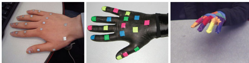
Fig. 12.2 Marker-based methods. Left the reflective markers used in [40]. Middle the color markers with different colors used in [32]. Right the color glove used in [36]
