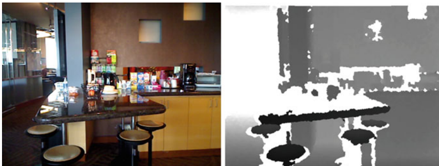
Fig. 1.12 Artifacts commonly occur in depth capture of natural scenes using commercial 3D cameras. Left RGB image. Right Depth map captured by the first-generation Kinect of the same scene. Pixels in white are holes in the depth map which arise due to specularities occlusion or clutter. Image courtesy [9]
