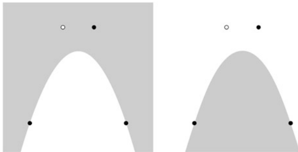
Fig. 2.6 An example of two cubic Bézier curves with control points (0, 0) , (b_0, b_1) , (2/3, 1) and (1, 0) (left: (b_0, b_1) = (1/3 + 0.01, 1) , right: (b_0, b_1) = (1/3 - 0.01, 1) , represented by hollow circles). The implicit representation flips orientation, despite only a small perturbation of the control points
