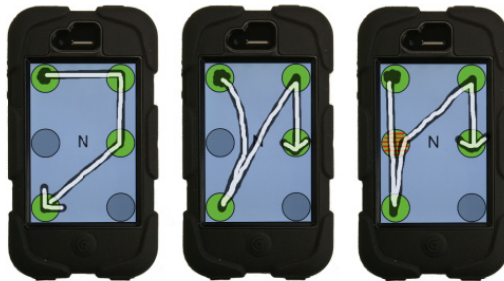
Fig. 1. Possibilities to enter the letter “N” with EdgeBraille. (a) Selecting the dots using the shortest path (b) Selecting the dots column wise circling around dot no. 2 (c) Selecting the dots by first activating dot no. 2 and then deactivating it on the way back from dot no. 3.
