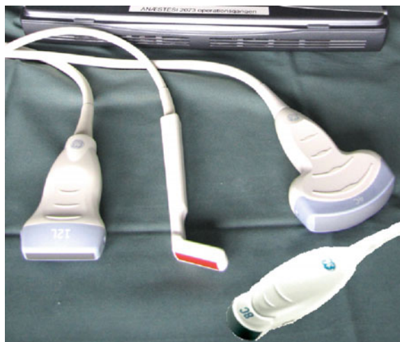
Fig. 16.1 Ultrasound transducers useful in airway management. Left Linear 7–12 MHz high-frequency transducer. Second from left Small linear 6–10 MHz high frequency “hockey stick” transducer. Upper right Curved, Convex 2–6 MHz low frequency transducer. Foreground, insert, micro convex 4–10 MHz transducer
