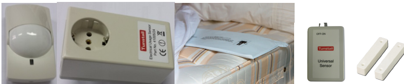
Fig. 2 Presence sensor, Electrical power consumption, Occupancy sensor, universal sensor, door contact
