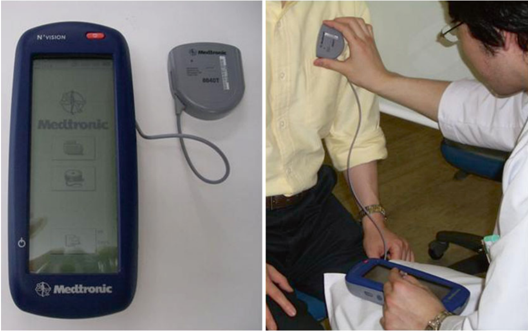
Fig. 5.12 The N V ision (model 8840, Medtronic Co.). The programmer is used to review and program device parameters. The programmer is also used to set limits for the patient control devices
