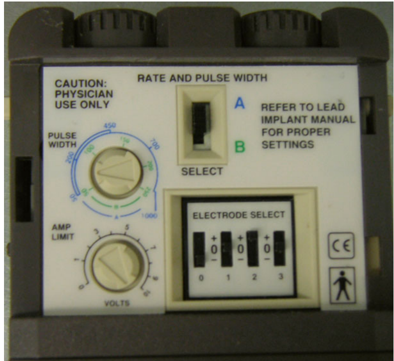
Fig. 10.5 Stimulation device for intraoperative test stimulation. This is gas-sterilized and controlled by the surgeon
