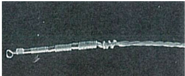
Fig. 5.3 The early DBS electrode (model 3380). This platinum-iridium electrode is composed of a distal loop and three other active contact points, each approximately 2-mm long
