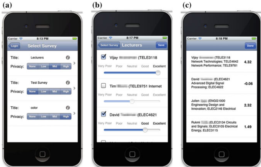
Fig. 4.3 Screenshots of iPhone app showing (a) list of surveys and privacy levels available to the workers, (b) the questions and ratings entered by the worker, and (c) the worker responses uploaded after noise addition
