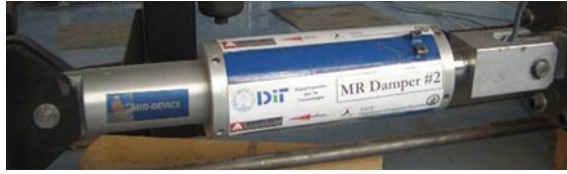
Fig. 13.7 One of the two prototype MR dampers
