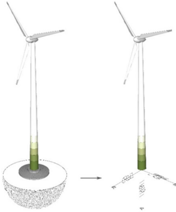
Fig. 12.3 Wind turbine model with soil springs for the soil–structure interaction influence
