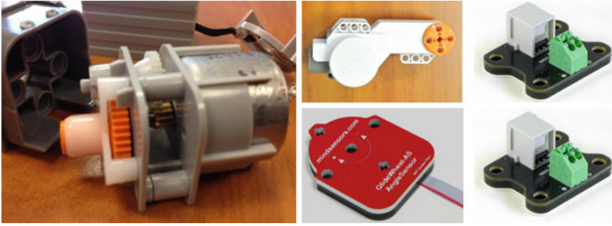
Fig. 14.7 a DC generator with gearbox (E-motor), b Actuator (NXT-motor), c Angle sensor (Glide-Wheel-AS), d CurrentMeter for NXT, e VoltMeter for NXT
