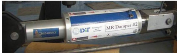
Fig. 13.7 One of the two prototype MR dampers
