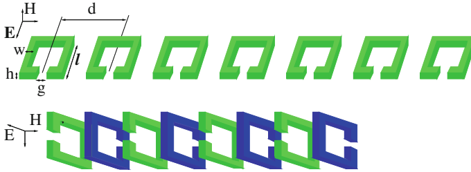
Fig. 14.1 Schematic view of a one-dimensional array of split-rings in ( upper ) the planar geometry; ( lower ) the axial geometry. The magnetic field is perpendicular to the planes of the rings
