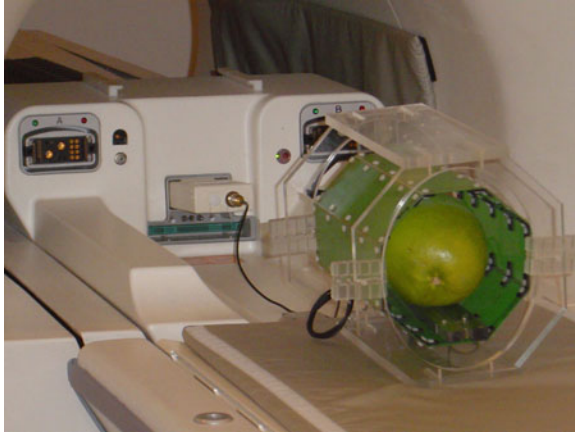
Fig. 3.11 Eight-element MI ring with a pomelo imaging subject in a clinical MRI scanner
