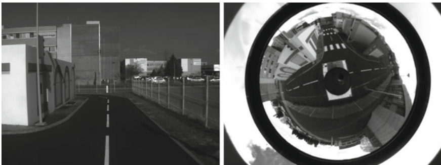
Fig. 1 Images from two mobile robots at the same place with different cameras, perspective ( left ) and omnidirectional ( right ). The points of view are not the same because of the pole supporting the omnidirectional camera
