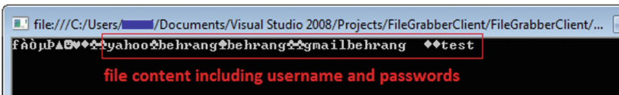
Fig. 6. Unauthorized access to PasswordWallet data file
