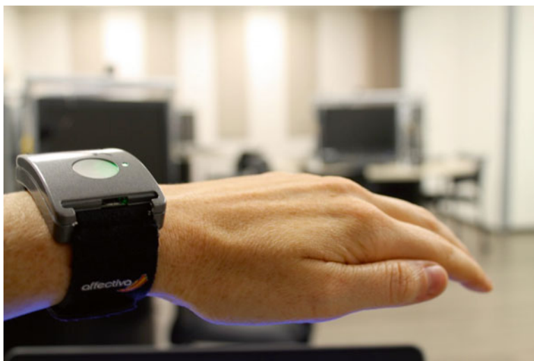
Fig. 10.3 Affectiva Q™ sensor is used to track electrodermal activity in dynamic environments
