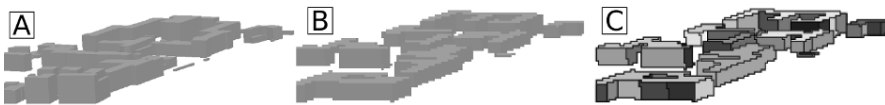
Fig. 17.7 Entropy of rasterised 3D scene: A) High resolution raster of original buildings; B) Normal resolution raster with generalised buildings; C) Vector polygon map of visible buildings' faces derived from B
