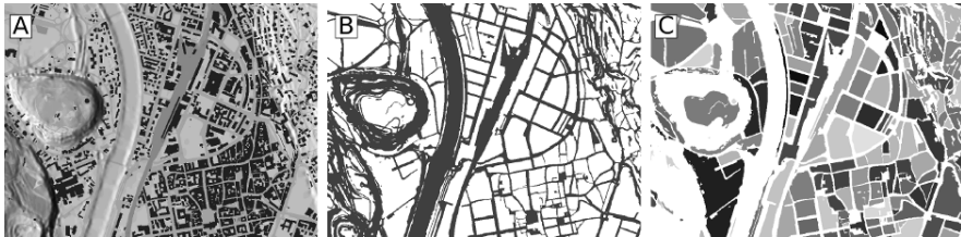
Fig. 17.1 A) Shaded landuse map of Trento and buildings; B) Non-nil pixel groups which split the city space into quarters (inverting pixel map); C) Final map of raw quarters (defining quarter areas having unique values)
