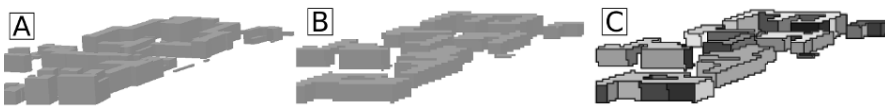
Fig. 17.7 Entropy of rasterised 3D scene: A) High resolution raster of original buildings; B) Normal resolution raster with generalised buildings; C) Vector polygon map of visible buildings' faces derived from B
