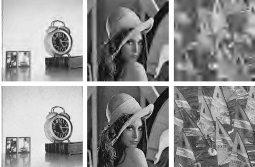
Fig. 14.1 Top row: Reconstruction by tensor-product wavelet compression using the 7–9 biorthogonal filter bank with 1,000 wavelet coefficients for test image clock (PSNR 29.93), 700 coeffs for Lenna (PSNR 24.28), and 200 coeffs for sail (PSNR 19.58). Bottom row: Reconstruction by EPWT wavelet transform using the 7–9 biorthogonal filter bank with 1,000 wavelet coefficients for clock (PSNR 33.55), 700 coeffs for Lenna (PSNR 30.46), 200 coeffs for sail (PSNR 27.19)
