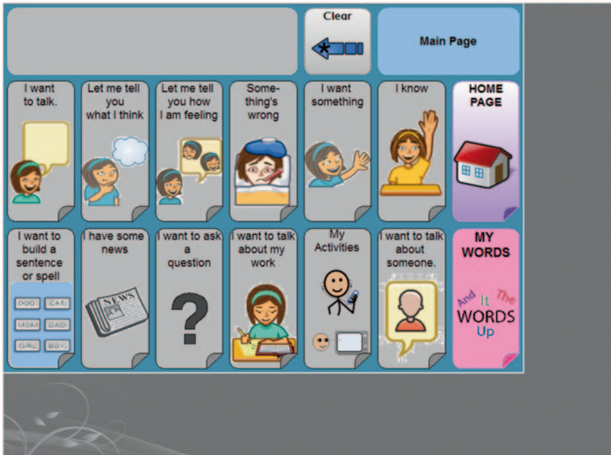
Fig. 23.15 Screenshot of Window view of Tobii Communicator with the height and width of the page-set set to 80% relative to the screens size and positioned in the top left corner of the screen. Page set properties feature in Tobii Communicator showing settings for reduced Window view with the docked position of 80% width and height in the top left corner of the screen. © 2013 Tobii Technology. (Photo of the screenshot: Judy Lariviere)
