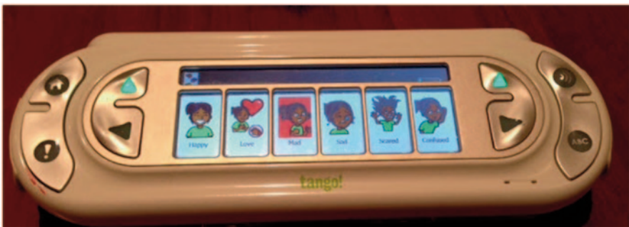
Fig. 23.9 Tango AAC device. The horizontally arranged six buttons in the middle of the device were activated through a touch display or screen. The arrows surrounding the screen supported navigation between the dynamic display screens for accessing additional vocabulary on the same topic and for changing topics. The outer buttons provided access to the home screen, alphabet, volume control, and PopTalk, which included high-frequency, quick phrases. (Photo: Judy Lariviere)
