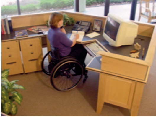
Fig. 24.5 Universal design features that provide flexibility, such as large workspaces that locate all objects within reach, enable easy access to all parts of a workstation and facilitate work tasks for individual workers and teams. These features illustrate principles: P1. Equitable use, P2. Flexibility in use, P3. Simple and intuitive use, P4. Perceptible information, P5. Tolerance for error, P6. Low physical effort, P7. Size and space for approach and use, P8. Social integration, and P9. Contextual integration
