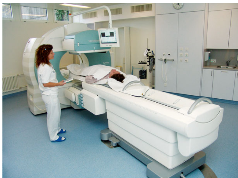
Fig. 31.1 Example of a hybrid SPECT/CT system consisting of a 16-slice CT and a dual-head gamma camera
