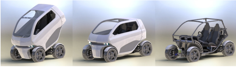
Fig. 1 Folding EOsc2 for reduced parking space and higher maneuverability
