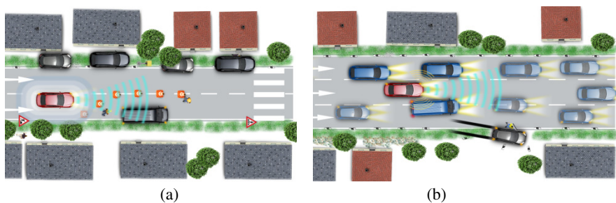
Fig. 5 Use-cases for the uNRA (ego vehicle in red): (a) Narrow passage caused by static surroundings, (b) Narrow passage caused by dynamic objects
