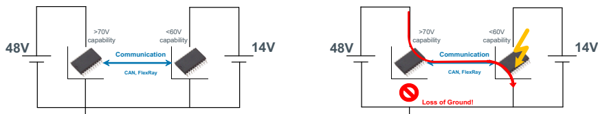
Fig. 2 Failure mode - loss of ground (left: no failure / right: loss of Ground at the 48V side)
