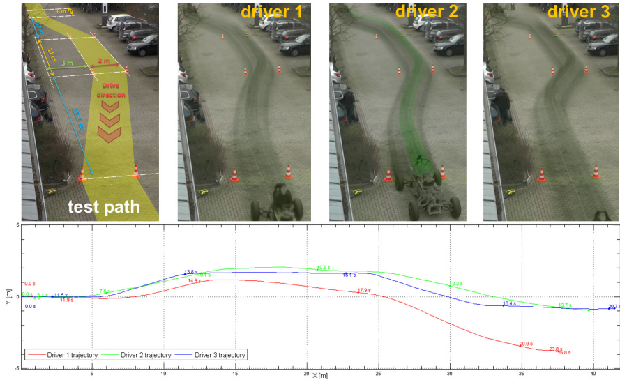
Fig. 6 Lane change experiments for three drivers and corresponding trajectories from simulation replay
