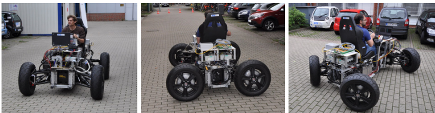
Fig. 3 Ackermann, sideways and turn-on-the-spot drive modes
