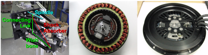
Fig. 2 Shock absorber connected to ride height changing spindle and the new motor housing
