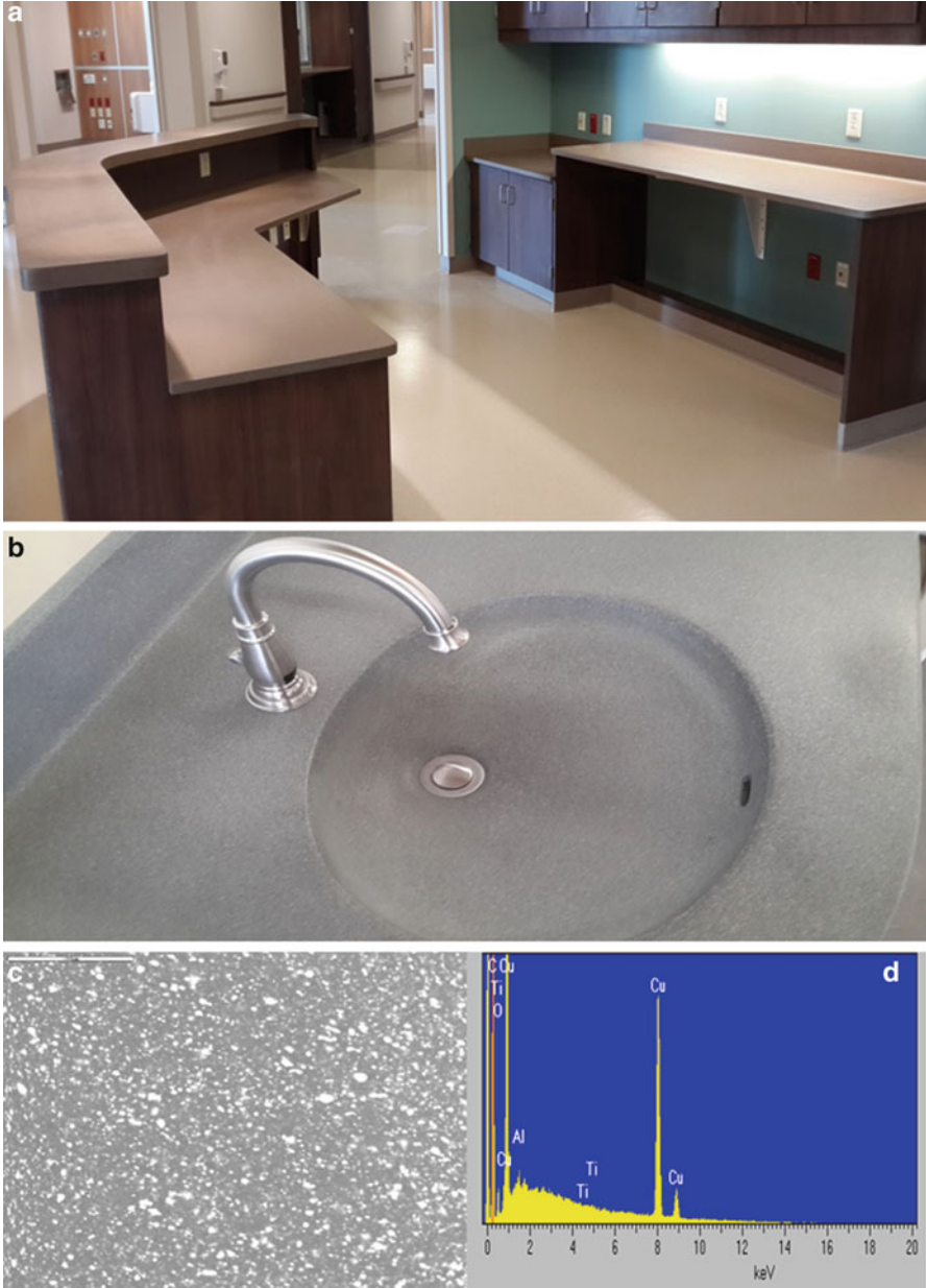
Fig. 5.4 Copper oxide impregnated non-porous surfaces. (a) A nurse top station in which the non-porous countertops are impregnated with copper oxide particles. (b) A sink made with non-porous copper oxide impregnated material. (c) SEM picture of the non-porous material shown in (b), demonstrating the homogenous distribution of the copper oxide particles on the material surface. (d) An X-ray photoelectron spectrum analysis of a white dot particle shown in (c), demonstrating the presence of copper
