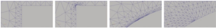
Fig. 5 Detection of genuine geometric singularities. Evolution of the initial upper-left corner of the deformable shape (see top of Figs. 3 and 4). The adaptive ASQP method is able to sort out whether geometric singularities are genuine to the problem or just due to lack of numerical resolution and to coarsen overrefined regions of the computational grid
