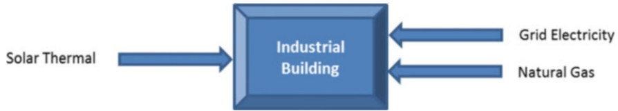
Fig. 2.11 Layout of energy resources for industrial building case study, when using solar thermal energy
