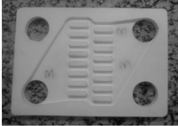
Fig. 6.10 Ceramic plate constructed with alumina using gelcasting technique
