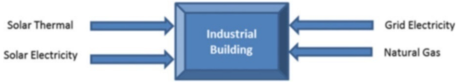
Fig. 2.14 Layout of energy resources for industrial building case study when using hybrid system
