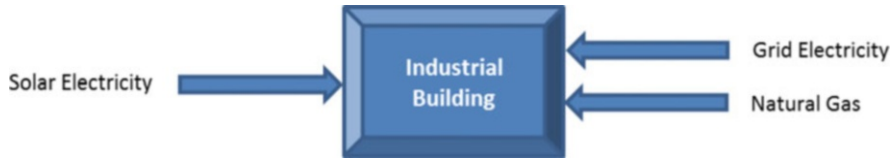
Fig. 2.12 Layout of energy resources for industrial building case study, when using solar electricity energy
