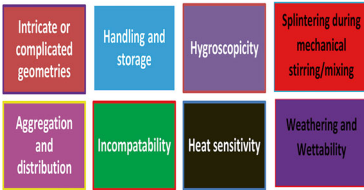
Fig. 5.8 Representing the challenges and technical problems faced during manufacturing of natural fibre composite
