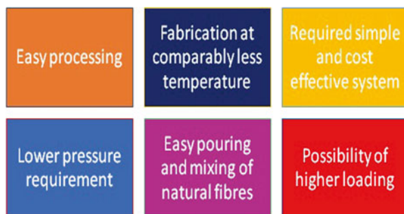
Fig. 5.4 Advantages of thermoset polymer for natural fibre-reinforced composites
