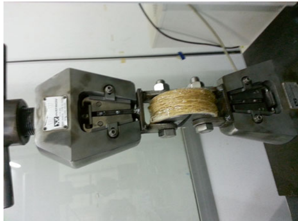
Fig. 18.5 Split-disk test for a filament wound kenaf composite specimen
