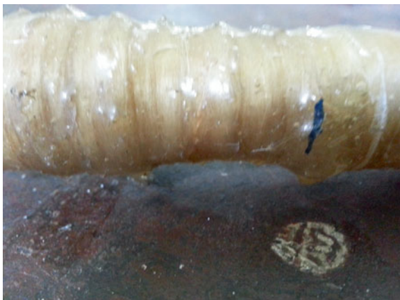
Fig. 18.6 Kenaf composite specimen in torsion test
