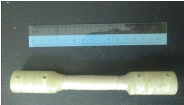
Fig. 18.3 Shaft made from filament winding process
