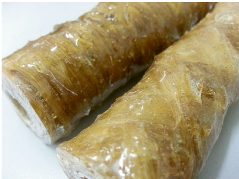
Fig. 18.13 Kenaf fibre composite hollow shafts fabricated using the improved method
