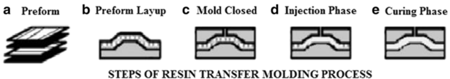
Fig. 13.1 Sequence of the main steps of RTM process. (a) realization of the preform, (b) deposition and draping of the preform in the mold cavity, (c) closing mold, (d) injection phase, and (e) curing phase
