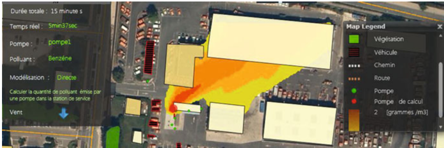
Fig. 2 Web services to view Benzene propagation around a gasoline station from fictive measures
