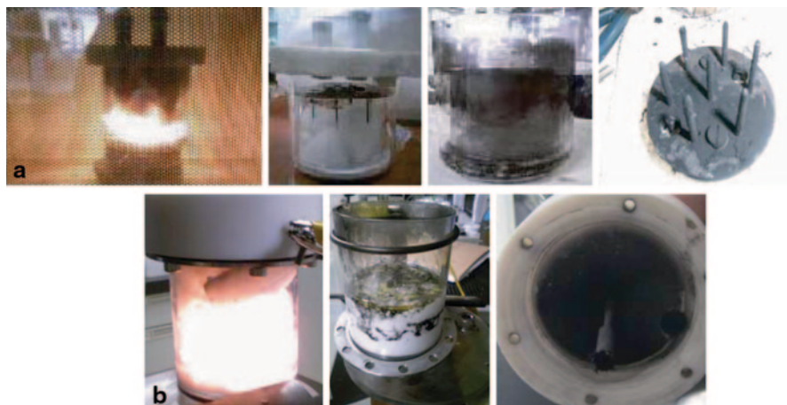
Fig. 30.5 Photo of the high frequency plasma decomposition of clathrate hydrates. a 2.45 GHz MW plasma decomposition. b 27.12 MHz RF plasma decomposition
