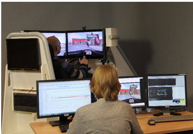
Fig. 1. Driving simulator with eye tracking in action
