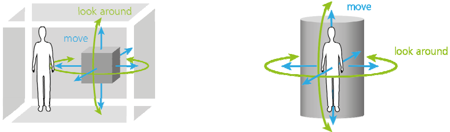
Fig. 4. Relations between object shape and usage in an immersive scenario: The axes of the cube are projected on the spatial axes of the virtual environment, whereas the cylinder is perceived like a simple pawn
