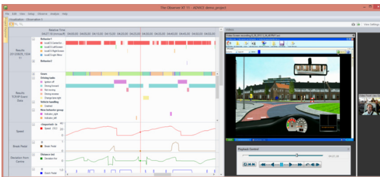
Fig. 2. The Observer XT: integrated display of the driver's main front screen with gaze overlay, gaze events (red colored bars), driving tasks (multi-colored bars), and vehicle parameters (red/green/blue lines)
