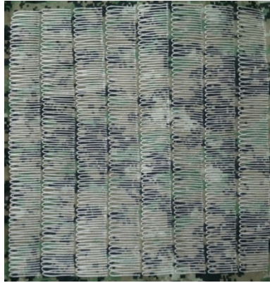
Fig. 2. A sample of an 8 x 8 flexible plastic optic fiber patch
