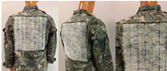
Fig. 3. A sample of flexible plastic optic fiber display (color off)
