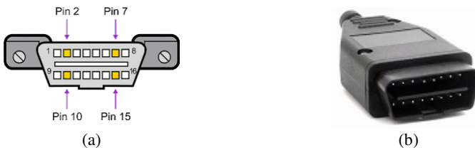
Fig. 3. (a) J1962 CAN/OBD-II 16-pin socket, (b) CAN/OBD-II DLC
