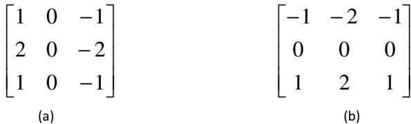
Fig. 1. Sobel operator. (a) is the operator along X direction while (b) is the operator along Y direction
