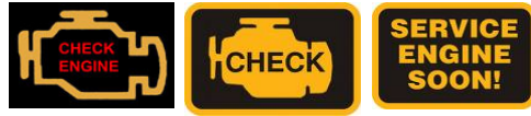
Fig. 1. Various symbols of MIL or the check engine light. (Pictures are copies from Ford, GM, and Toyota vehicle maintain manuals).
