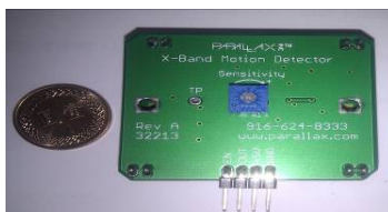
Fig. 5. X-band motion detector
