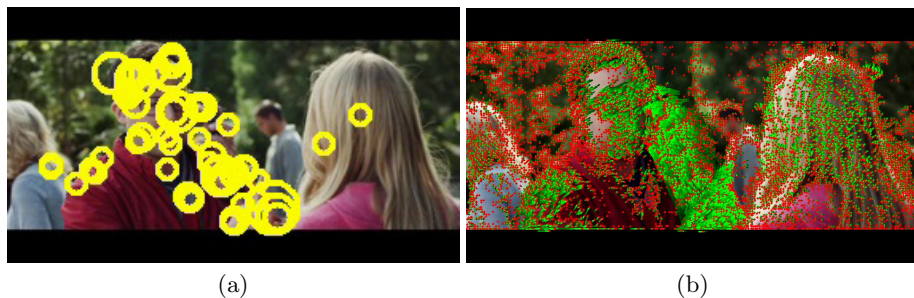
Fig. 2. Local video locations of interest: a) STIPs and b) video frame interest points tracked in consecutive video frames
