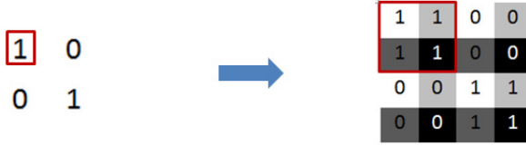
Fig. 1. Interleaving coded aperture (a grayscale indicates a sub-mask)
