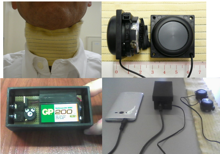
Fig. 4. EL transducer, amplifier and entire system (upper left: EL transducer with neck-bandage, upper right: a pair of EL transducer, lower left: amplifier in a box, lower right: entire system)
