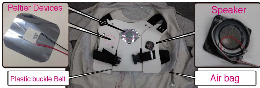
Fig. 2. The Configuration of wearable system to present tactile sensations as pseudo heart-rate, body temperature and chest pressure
