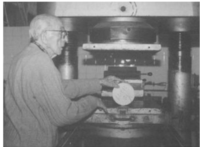
Fig. 13 Prof. Carneiro at the laboratory preparing a sample for the Brazilian test (after Fairbairn and Ulm 2002)
