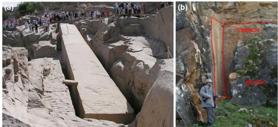
Fig. 6 Rock column or block extraction techniques in Egypt and Anatolia: a slots around the unfinished obelisk in Aswan (Egypt) (Hamada et al. 2004), b slots around a marble block in Aphrodisias (Turkey) (Kumsar et al. 2003)
