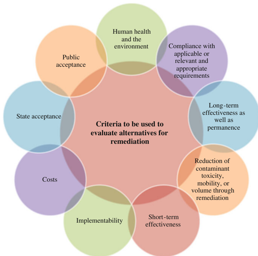
Fig. 1 Suggestions of Environmental Protection Agency (EPA) in order of preference that the nine criteria may be used to evaluate alternatives for remediation
