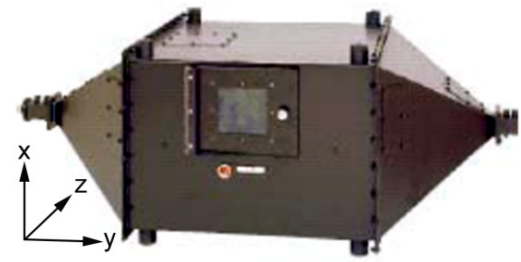
Fig. 2 TEM cell and the coordinate system
