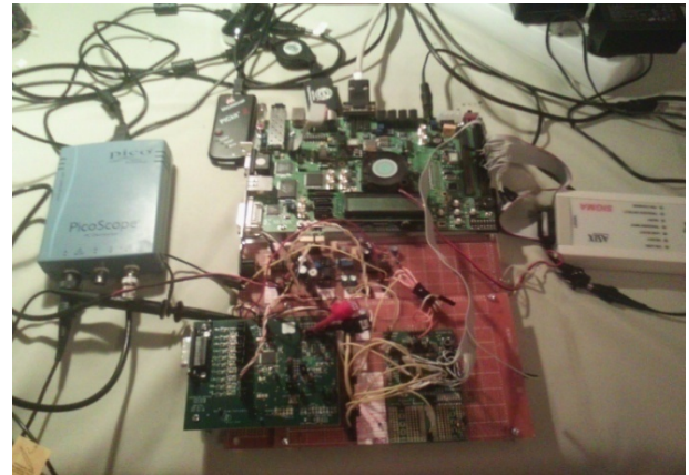
Fig. 6 Connecting Xilinx XUPV5 board to ADS1298 [12]
