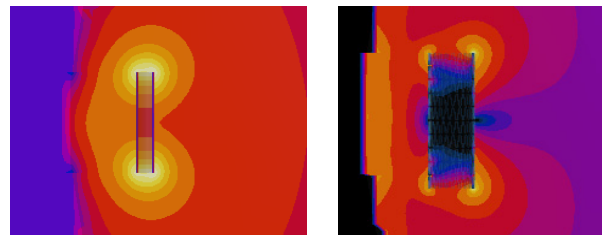
Fig. 1 Temperature distribution around a cylindrical stent, when exposed to an 835 MHz EM radiation[5]
