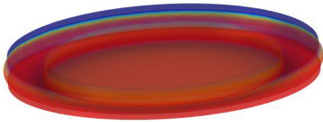
Fig. 2 PZT deformation, magnified 3e7 times for better viewing
