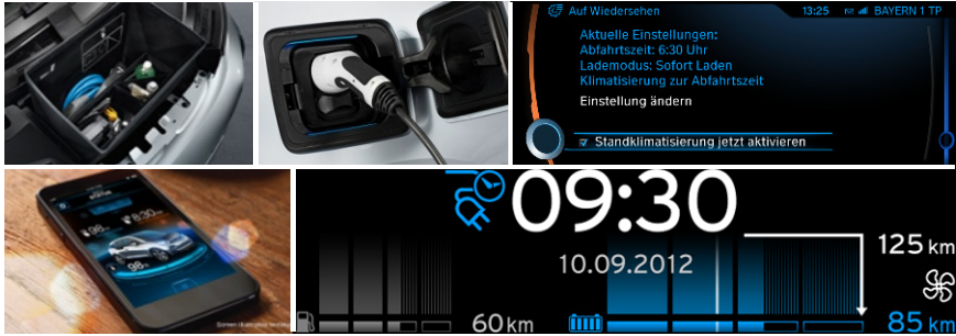
Fig. 9. Charging features of BMW i3 (Fotocredit: BMW Group / A0145735.). Top: Cable box under the bonnet, illuminated socket, Goodbye Screen. Bottom: BMW iRemote App, charging screen (range extender version).
