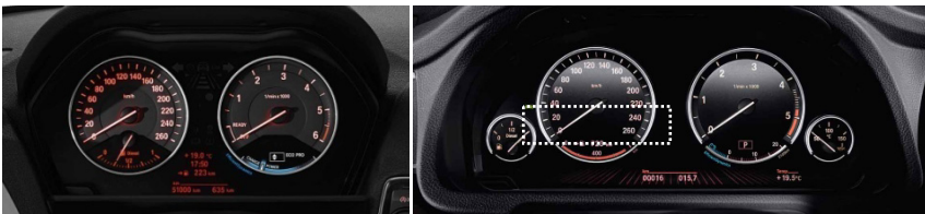
Fig. 1. BMW heritage (Fotocredit: BMW Group): The current “two eyes” (F20 1 series, left / A0161657) and “four eyes” (F10 5 series, right / A0173684) cluster instruments. Dotted line (right) indicates the display size of the BMW i3 cluster instrument display in comparison.
