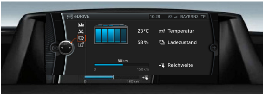
Fig. 8. Removed iDriveMenu “eDRIVE” BMW ActiveE (Fotocredit: BMW Group / A0145735.): Battery Info including Battery Temperature, SoC, and Range.
