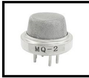
Fig. 4. MQ-2 gas sensor for flammable gas
