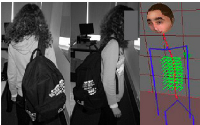
Fig. 4. Adopted posture for carrying an ordinary backpack using one of its handles and the resulting HARSim simulated model (left and right side respectively)
