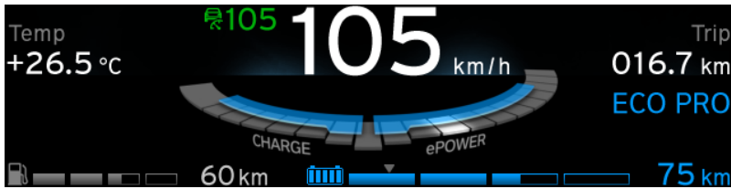
Fig. 2. Cluster Instrument BMW i3 (Fotocredit: BMW Group): Display area with current speed, drive train gauge, fill levels and ranges for petrol (range extender version) and battery. Top left on board computer (toggle). Top right Trip. Green speed indication: Current speed = ACC or DCC resume speed. ECO PRO: Current mode).
