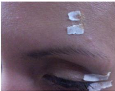
b) Eyebrow up closing the circuit.
