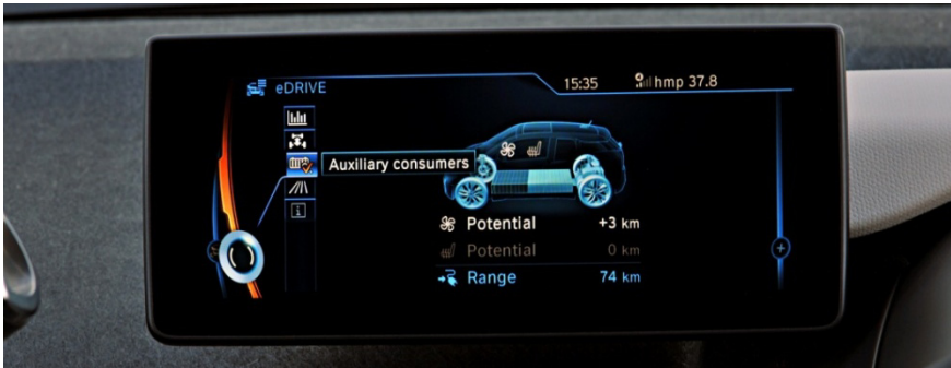
Fig. 7. NewiDriveMenu “eDRIVE” BMW i3 (Fotocredit: BMW Group): Auxiliary Consumers. Seat heatings are turned off, so no range potential is displayed.
