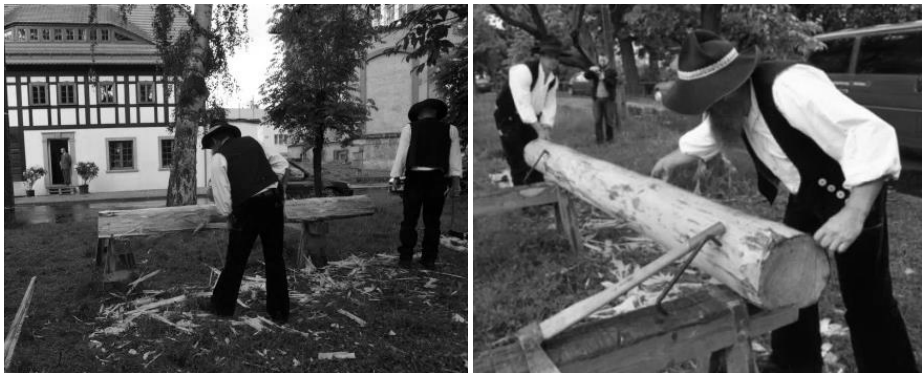
Fig. 12. Open Day of Half-Timbered Homes, Bogatynia – popularization of the craft of joinery and a presentation of log carving for log walls (photos by E. Trocka-Leszczynska, 2010)
