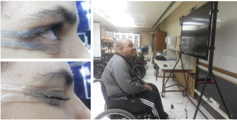
Fig. 5. Winkymote, an infrared-controlled interface for individuals with quadriplegic disability
