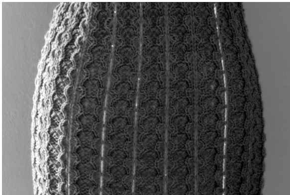
Fig. 5. The optical fibre fitted to the sub structure of the knitwear
