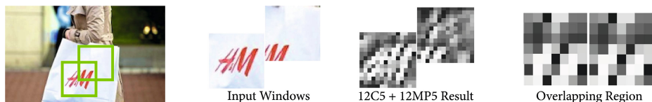
Fig. 4. Two adjacent windows extracted from an input image, passed through the 12C5 + 12MP5 feature extractor. A detailed view of the convolved maps in the overlapping region shows that these areas fully match.
