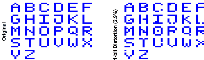
Fig. 6. Character patterns used in the second recognition test using RF-DHGN for all characters with 2.90% distortion
