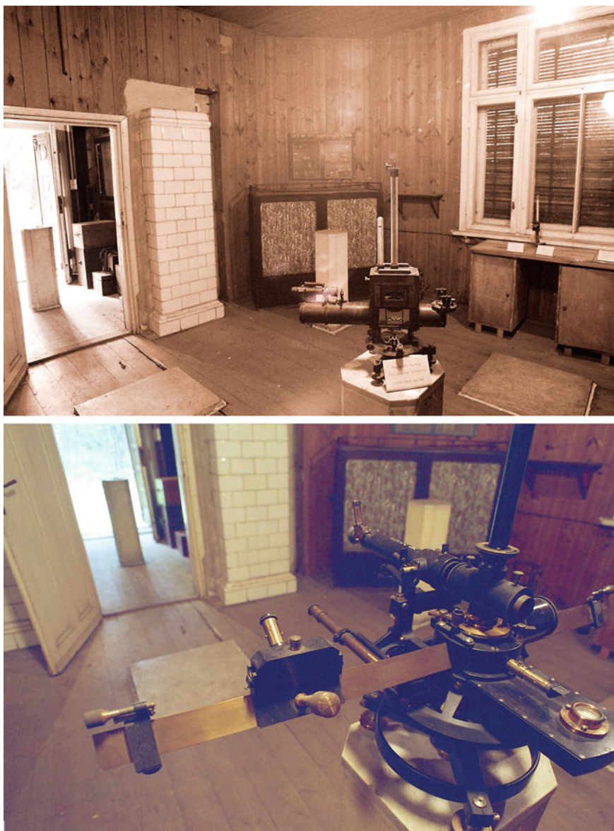
Fig. 1 Some of the modern instruments installed in the 1920s at the newly-built Świder Observatory. Top The Kew magnetometer of the Cambridge Scient. Instr. Co. Bottom The Sartorius magnetometer for magnetic declination measurements. Photos taken in the observatory museum by K. P. Teisseyre in 2006
