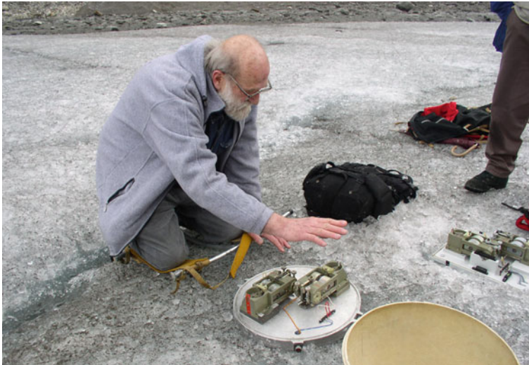
Fig. 8 Marek Górski at the Pasterze Glacier, Austria, 2006. Installation of micro-array of seismographs for tilt oscillation measurement. Photo by K. P. Teisseyre
