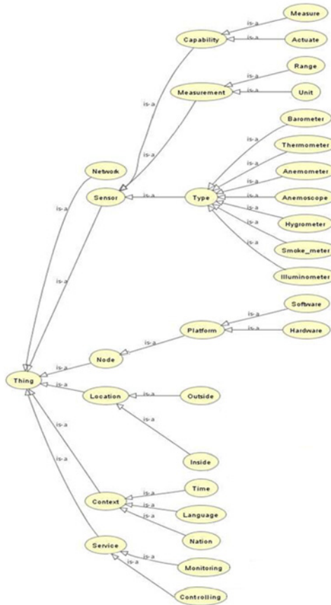
Fig. 2. Intelligent Control Service OWL-Model(Class) for the Proposed System
