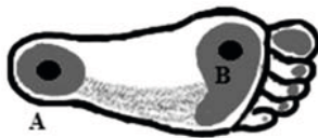
Fig. 3. Force sensors location on the foot
