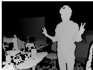
Fig. 5. Example of the depth image using infrared radiation
