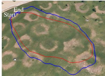
Fig. 3. Trajectories registered in one experiment projected over a satellite map: user (red line) and robot (blue line)
