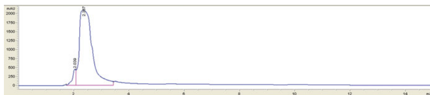
Fig. 11.5 Lactic acid peak obtained from HPLC analysis
