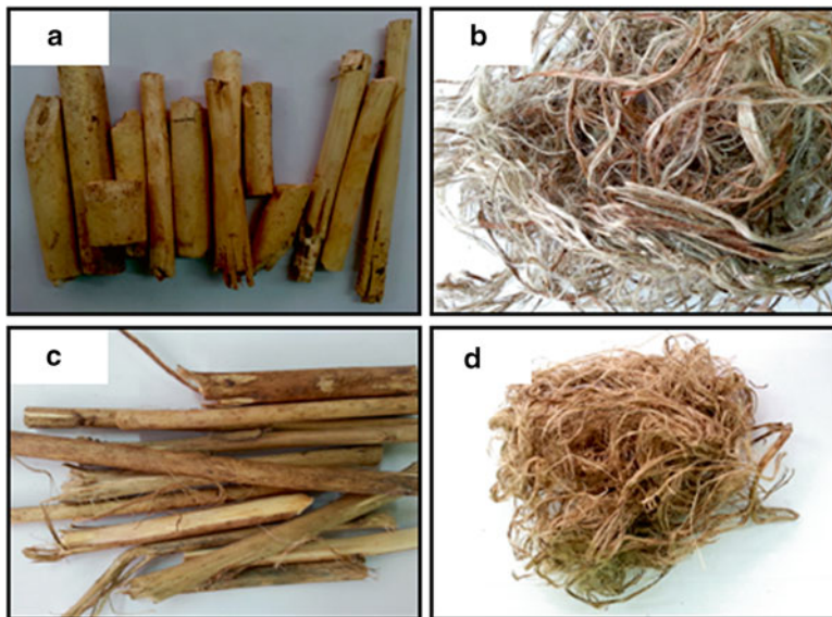
Fig. 1.11 Kenaf biomass: (a) Core; (b) core fibers; (c) bast; (d) bast fiber
