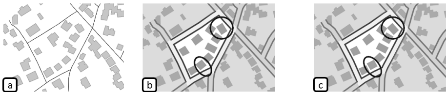
Fig. 5. (a) non-generalised data, (b) generalised data in 1:25k, using AGENT (only the central block was generalised), (c) generalised data using our PADAWAN modelling with buildings aligned to the road
