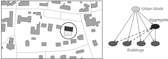
Fig. 2. Two adjacent buildings compose an aggregate. Aggregated buildings need to have normal interactions for buildings, but the aggregate also needs to interact as a whole.
