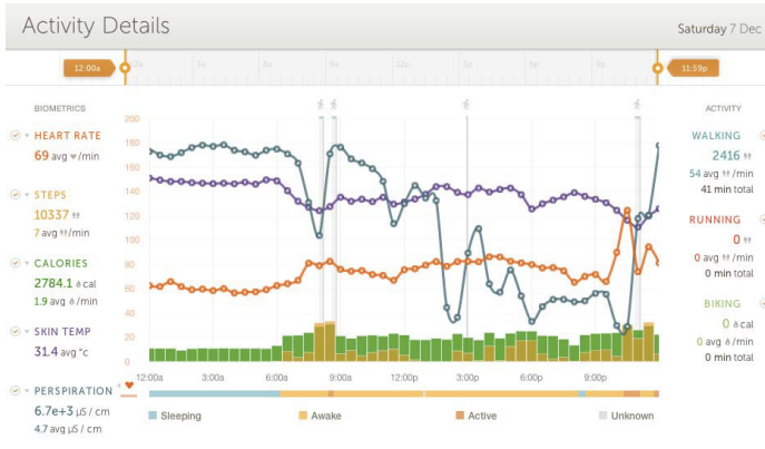
Fig. 5. The Basis Activity Details visualization allows the user to explore the relations between multiple biometric time series data (heart rate, steps, calories, skin temperature, perspiration, and activities) in an adjustable time interval
