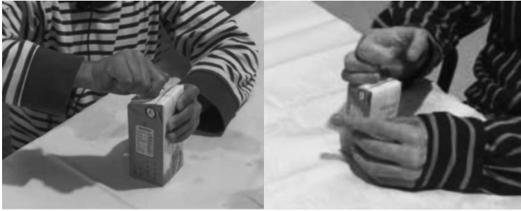
Fig. 7. Test of a child (left) and an adult with reduced hand function (right) opening package B, Tetra Brik® Aseptic 200 Edge with Helicap™ 23
