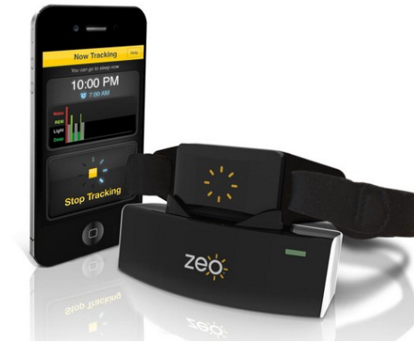
Fig. 2. Zeo sleep manager with electrode headband, base station and smartphone running the associated application
